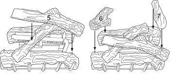
Figure 44 - Installing Log No. 5
